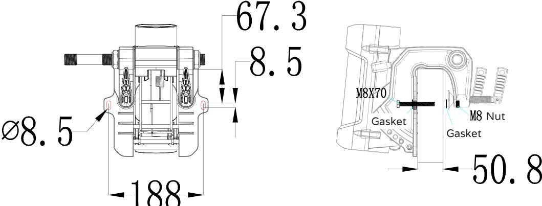
In order to avoid over-tightning thumb screws to prevent motor from dislocating, drill two screw fixing holes on the side of the boat according to the positions of the two screw holes on the left and right of the bracket (pictured on the left), and fix them with screws.
